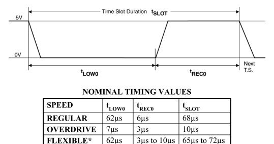
\*Powerup defaults for Flexible speed:  $t_{REC0} = 7\mu s$
