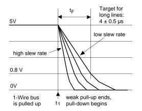
Extensive tests have shown that 1-Wire networks with lengths of up to 300m will perform best if the fall time  $t_F$  is in the range of  $4 \pm 0.5 \mu s$ . This translates into a slew rate of approximately  $1V/\mu s$ . This slew rate is typically achieved by selecting a PULLDOWN SLEW RATE parameter code of 0 x 4 (see MODE COMMANDS). If the actual measured fall time is longer than the target value, a parameter code of 0 x 3
